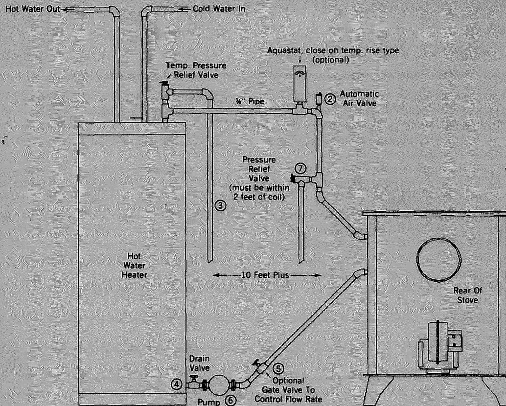
To install the optional hot water coil, Two holes will need to be drilled or cut into the side of the stove. There is a template for the hole location(s) that is included with the coil. Keep the holes above the firebricks and toward the back of the firebox. This location is best to not interfere with loading.
