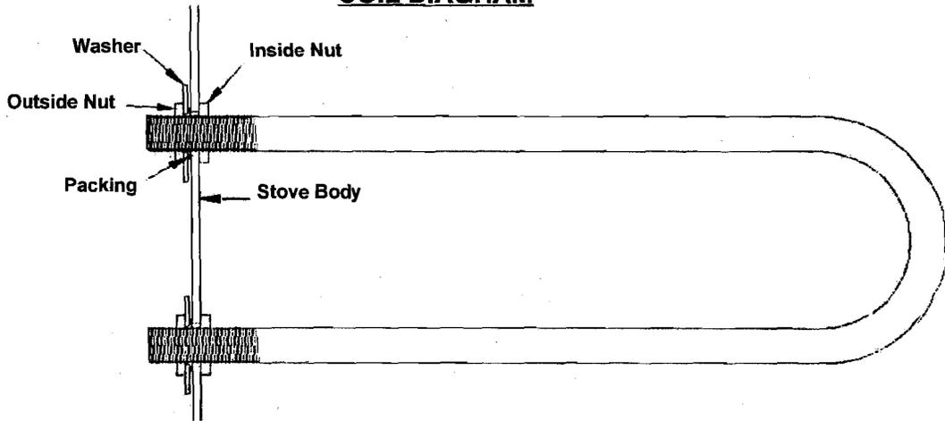
**PLUMBING DIAGRAM FOR THERMO-SIPHON METHOD - MAX. DISTANCE 10 FT.**
