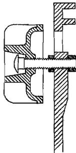
Next, lay the glass frame face down on a flat surface. Place the glass panel into the frame, making sure the gasket is only applied to the ends of the glass. Now by placing the door onto the frame, you'll see the holes will line up with the threaded holes in the glass frame. Using 4 flange-head bolts from the kit, tighten the glass frame onto the door.
