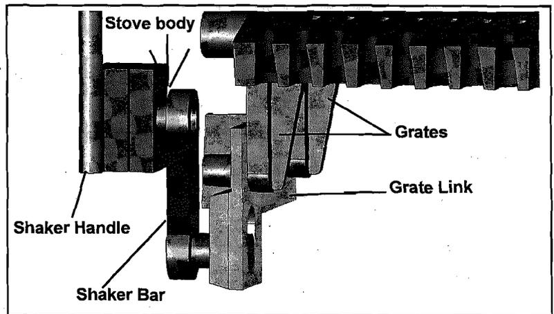
last forever, as long as you keep your ashes cleaned out of the stove. When ashes are left pile-up against the grates, the air-flow is blocked. With no air flow through the grates, they will begin to sag from the intense heat.
