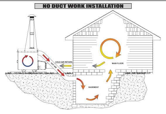
Cold air return must be installed in all installations, even those without an air duct system. If you do not, the furnace will not be able to heat the home. A filter should be installed in the cold air return. Furnace filters should be checked and cleaned/replaced regularly.
