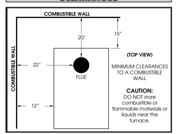
Sides of furnace, 12"; Rear of furnace, 15" (allow approximately 20" for the return box); Front of furnace, 36"; Heat Duct, 2" for the first 9 feet then 1" thereafter.
