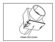
Figure 18.3 - Rear Vent Adapter
