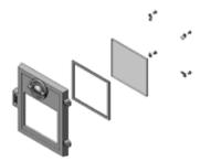
1. Lift the door off the hinges and place it face down on a sheet of cardboard or other nonabrasive fabric.
