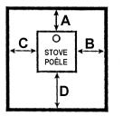
FLOOR PROTECTOR MUST BE NON-COMBUSTIBLE MATERIAL. IT MUST EXTEND BENEATH HEATER, AND TO THE FRONT/SIDEES/REAR AS INDICATED.
