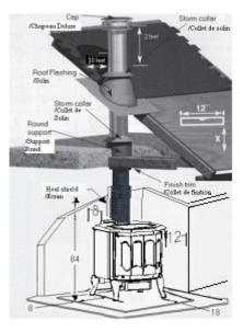
The *Vulcain* wood appliance must be installed in accordance with the applicable local laws or the CAN/CSA-B365, NFPA211 (USA) norms. Install the chimney following the manufacturer's instructions.
