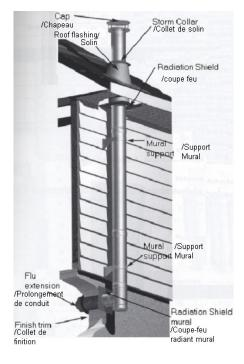
The *Vulcain* wood appliance must be installed in accordance with the applicable local laws or the CAN/CSA-B365, NFPA211 (USA) norms. Install the chimney following the manufacturer's instructions.
