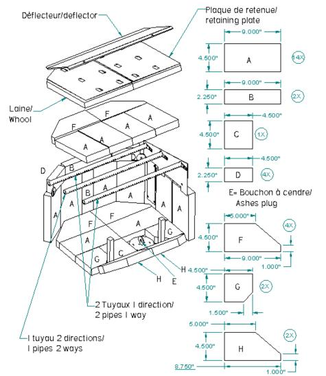
Place the firebricks as illustrated. They are identified by the letters A to H and the seal is cap identified by the letter E.
