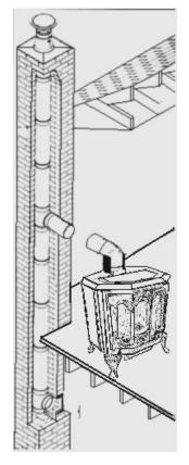
The *Mystere* wood appliance must be installed in accordance with the applicable local laws or the ULC S635, ULC S640, NFPA211 ( USA ) norms. Install the chimney following the manufacturer's instructions.
