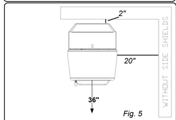
**Floor Protection: Front and side requirements are measured from the firebox opening. Floor Protector minimum: 25\" wide x 33\" deep.**
