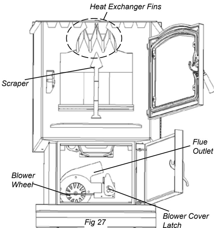
Whenever wood is burned, there is a potential for creosote formation. The venting system should be inspected periodically during the heating season to determine if a creosote buildup has occurred. If a significant layer of creosote has accumulated (3 mm or more), it should be removed to reduce the risk of a chimney or venting system fire.
