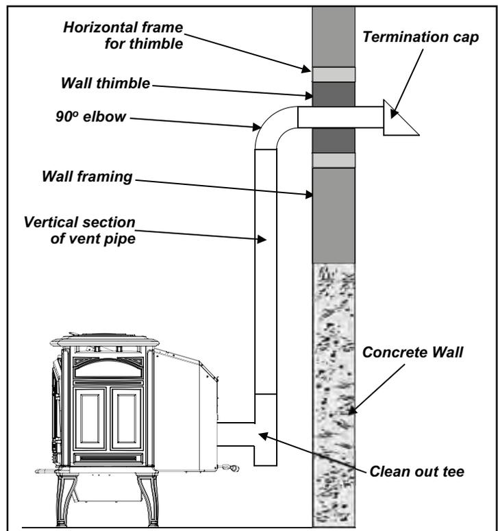
Figure 14: Venting with concrete wall behind unit .
