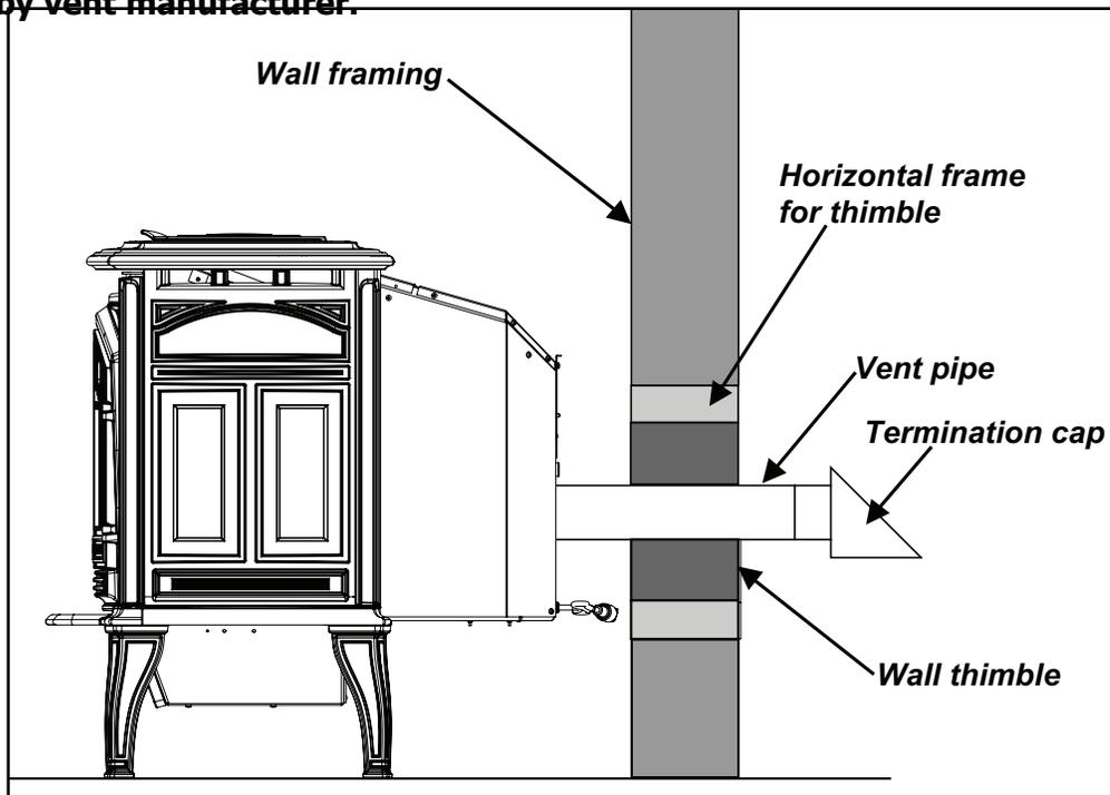
Figure 12: Straight through Wall Installation - Side View.
