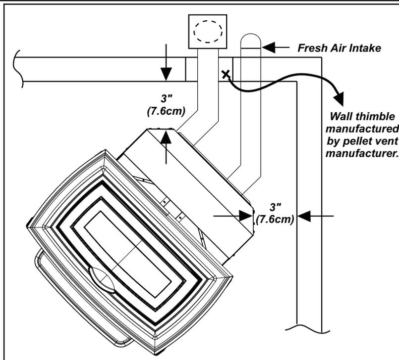
Figure 10: Corner Installation.
