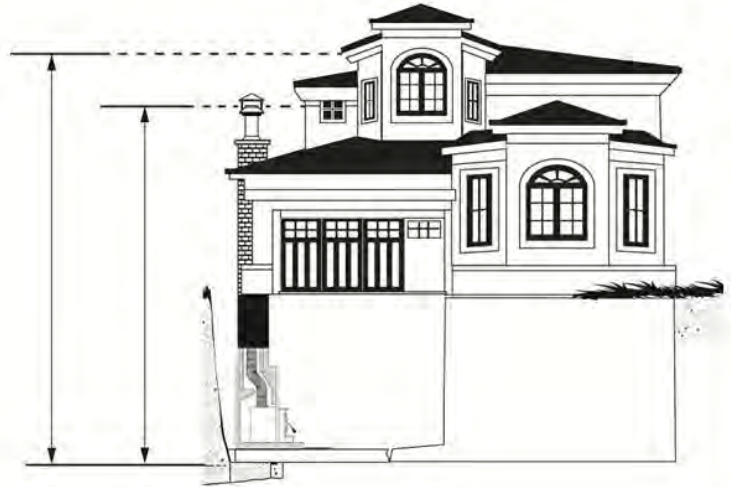
Figure 34: Chimney location in the house
