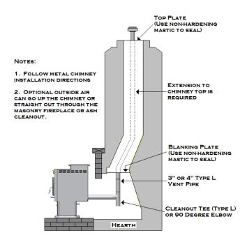
Measure and build chimney top plate. Cut out holes for chimney pipe, and if used the outside air pipe. Install and seal with non-hardening mastic to prevent water leakage. Install vent cap.
