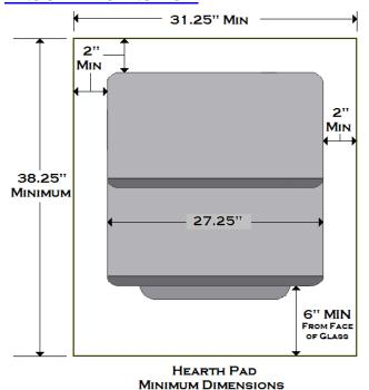
Freestanding installations require a minimum 33 ¼" wide by 36" long floor protection. The stove must be placed on a continuous (grouted joints) noncombustible material such as ceramic tile, cement board, brick, 3/8" millboard or equivalent, or other approved or listed material suited for floor protection.
