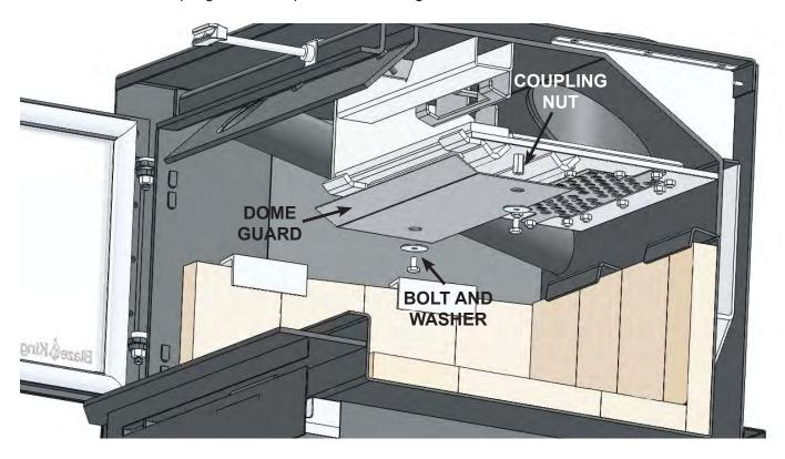
6. Remove the fourteen remaining 1/4-20 nuts from the dome bottom as well as the bypass shield. Lift the bypass door gasket retainer assembly upwards (enough to clear the threaded posts from the dome) and remove through the combustor opening. Once removed, ensure all debris is cleared from the inner surface of the dome.
